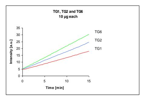
Please notice that the Transglutaminases used display significant differences in fluorescense intensity. However, all purified Transglutaminases discribed can be assayed using A101. The concentration of A101 in the assay is  $93 \, \mu g/ml$ .
