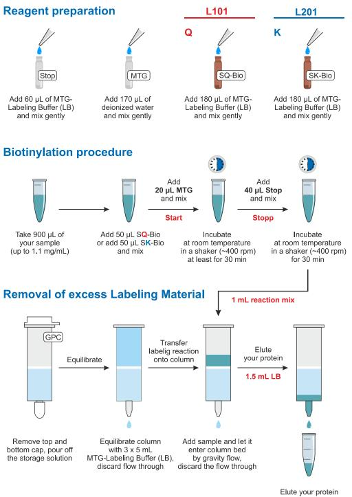
Elute your protein by adding 1.5 mL MTG-Labeling Buffer (LB), collect flow through
