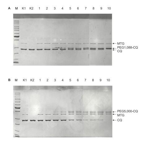
Figure 10: MTG mediated incorporation of PEG derivates into CQ.
