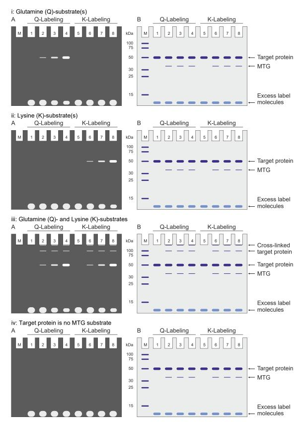
Figure 4: Schematically depicted results of Substrate Finder Kit. A = UV-illuminated gel; B = Coomassie stained gel; M = Protrein Marker; 1-4 = Labeling of free glutamine residues with SQ (timepoints 0 min, 5 min, 30 min, 60 min; 5-8 = Labeling of free lysine residues with SK, timepoints respectively.
