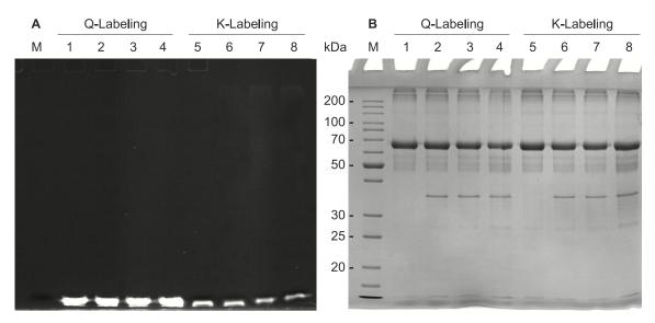
Figure 8: Labeling of Bovine Serum Albumin. A) UV-illumination of dansyl-residures and B) Coomassie stained SDS-PAGE-gel. M = Protein Marker; 1-4 = Q-Labeling, samples taken at 0 min, 5 min, 30 min and 60 min; 5-8 = Q-Labeling, samples taken at 0 min, 5 min, 30 min and 60 min.
